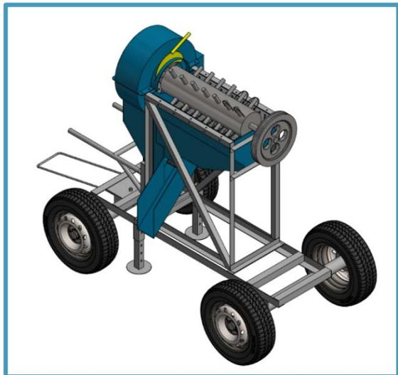
*The thresher design features easy-to-use controls and the machine can be transported by bicycle. Image credit: SIL*
